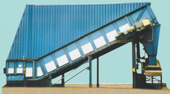
TUS Truck Unloading Station
